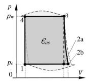
Figure 5: Indicator diagram of useful energy.
