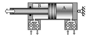
Figure 2: Schematic view of a suction-pressure unit [13].
