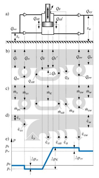
**Figure 3:** Suction-pressure unit: a) functional diagram, b) band chart of volume flux, c) band chart of mass flux, d) band chart of energy, e) pressure change.
